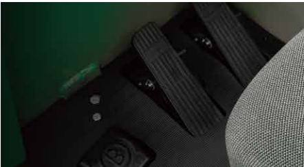
The safety pedals eliminate the safety hazard arising from the operator's incorrect operations.
